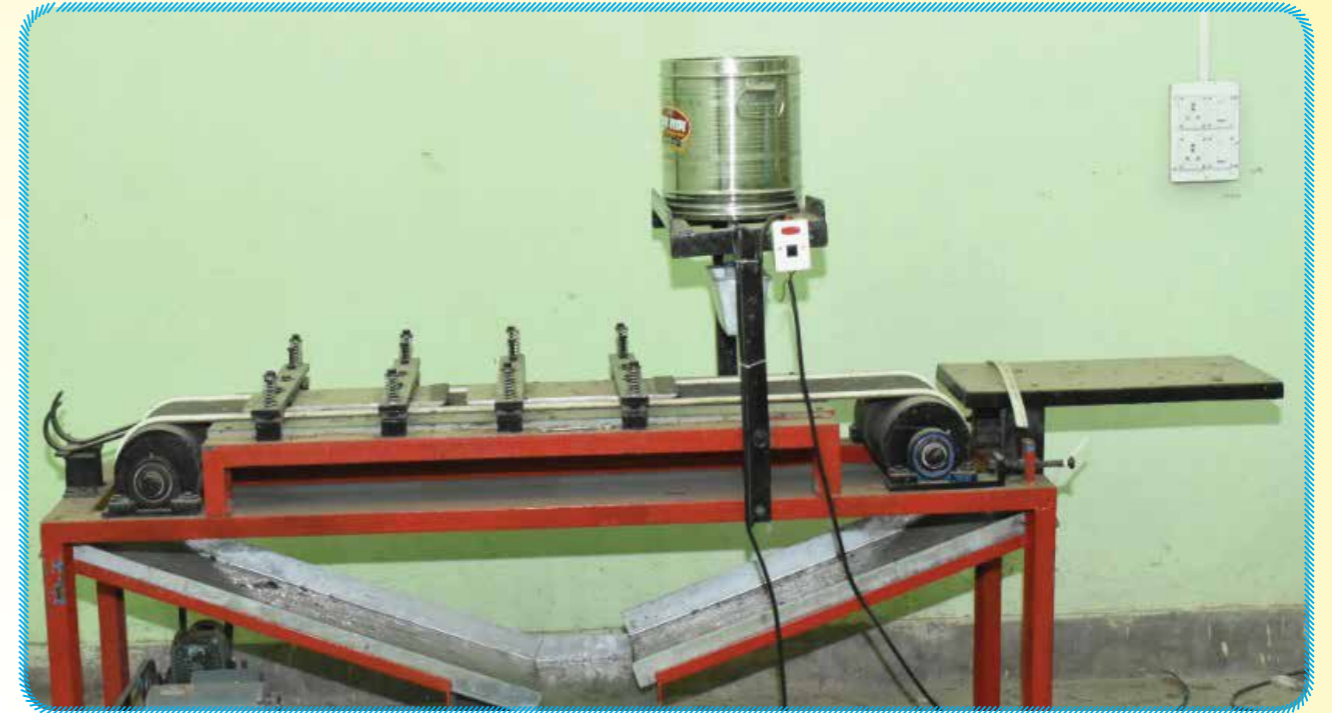
In-house Pencil-making machine (from waste paper)
