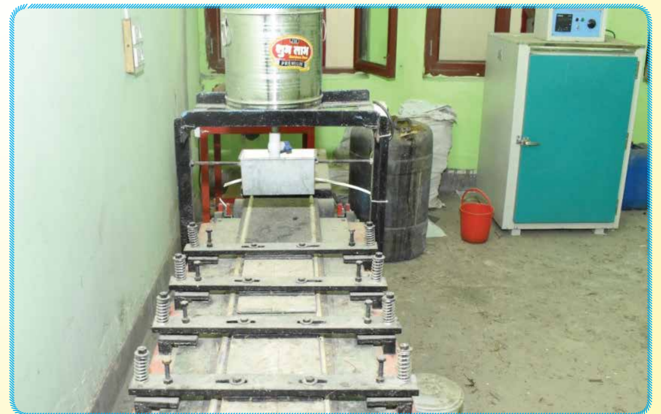
In-house pencil making machine and oven (from waste paper)
