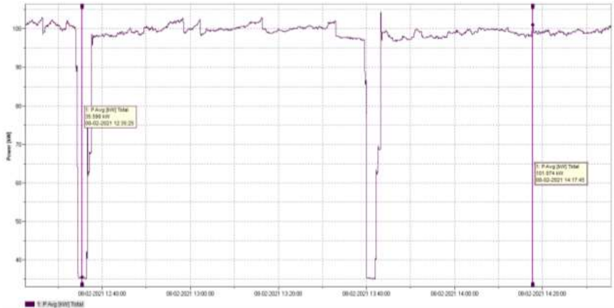
Power consumption pattern of Heat Pump- 3
