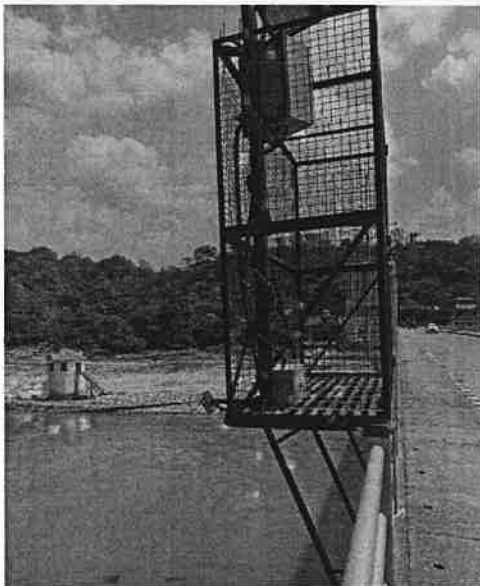
Photo 2- Early flood monitoring devices on the river Beas.
