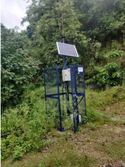
Photo 1- Early flood monitoring devices at Neugal Khad
