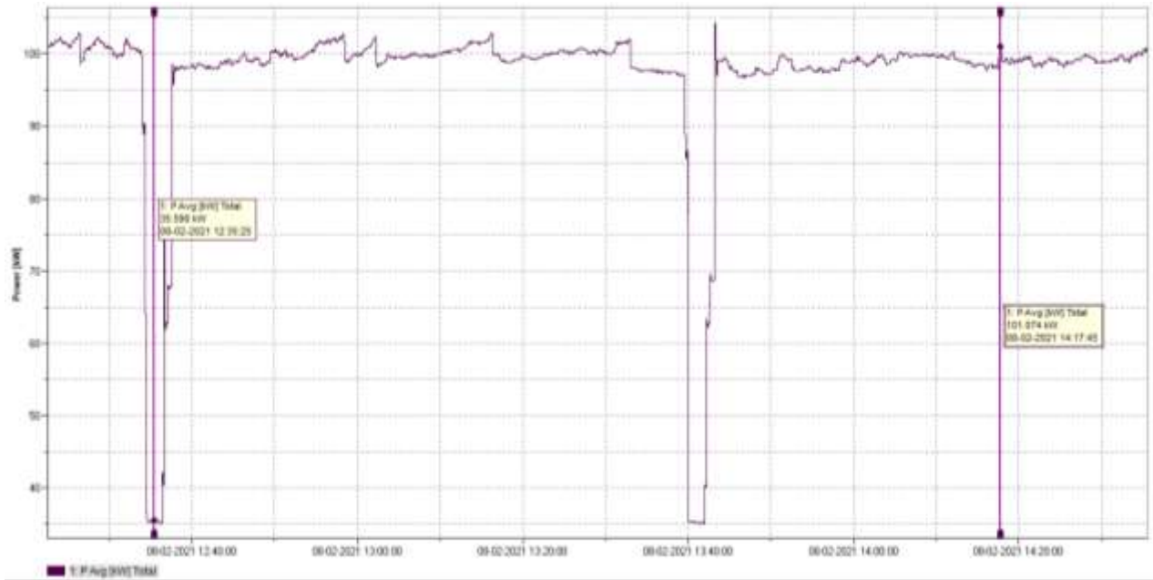
Power consumption pattern of Heat Pump- 3
